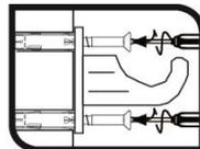
If recessed support brackets are required during building work, position the support bracket when cement is fresh and wait for it to set.
