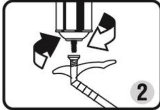
2. Remove the protective cap and screw the adapter. Hold the can upside down and activate the foam by pressing the valve
