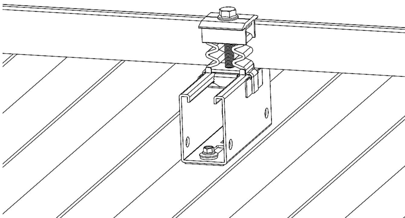
Application example 1: Direct fixing by thin sheet screws to a 2-ribs sandwich panel with flashing.
