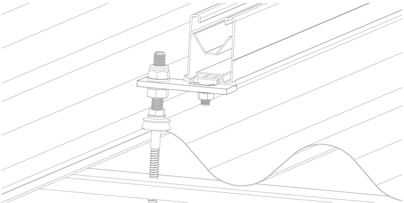
**Application example 2: Mounting of the PSE-A profile on KFS-AU**
