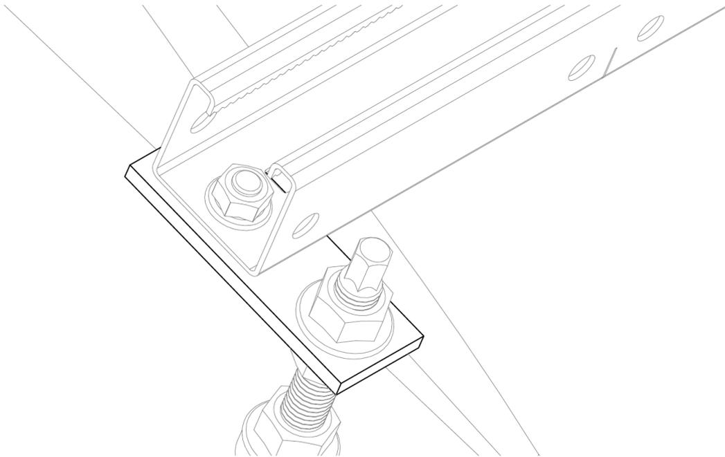
**Application example 1: Mounting of the GP-XS guide on KFS-RV**
