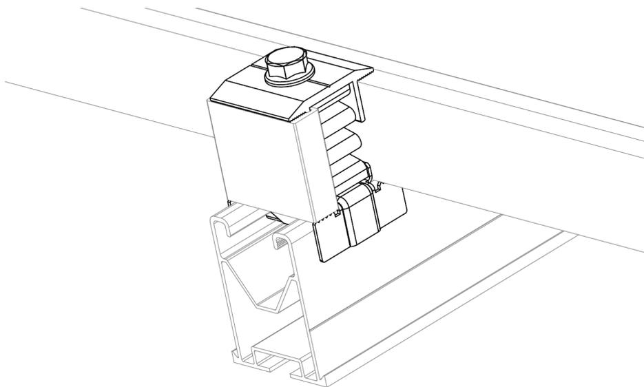
Application example 2: Mounting on a PSE-A “Aluminium profile for assembled fixing”
