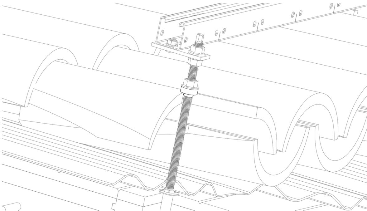
**Application example 2: assembly on sandwich panel roof and wood structure.**
