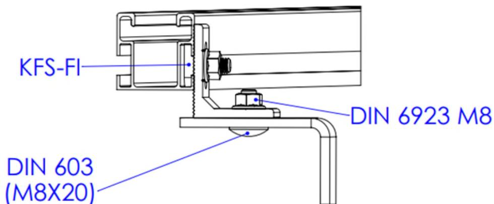
Application example 2: mounting of the PSE-C profile on roof hooks for curved tiles.
