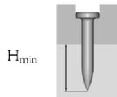
Installation depth ( $H_{min}$ ) in Concrete/ Steel
