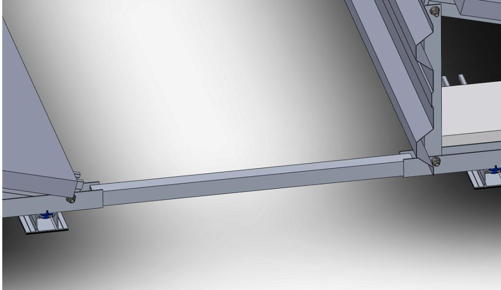
Fix the joining profile to the lower profiles by installing 2 stainless steel self-drilling screws on each side. The screws must be installed on the sides of the profile, in the shape of a cross so that they do not collide with each other. For the installation of the screws, an electric screwdriver equipped with a SW-8 hexagonal socket is needed, an installation speed of 1800 rpm is recommended.
