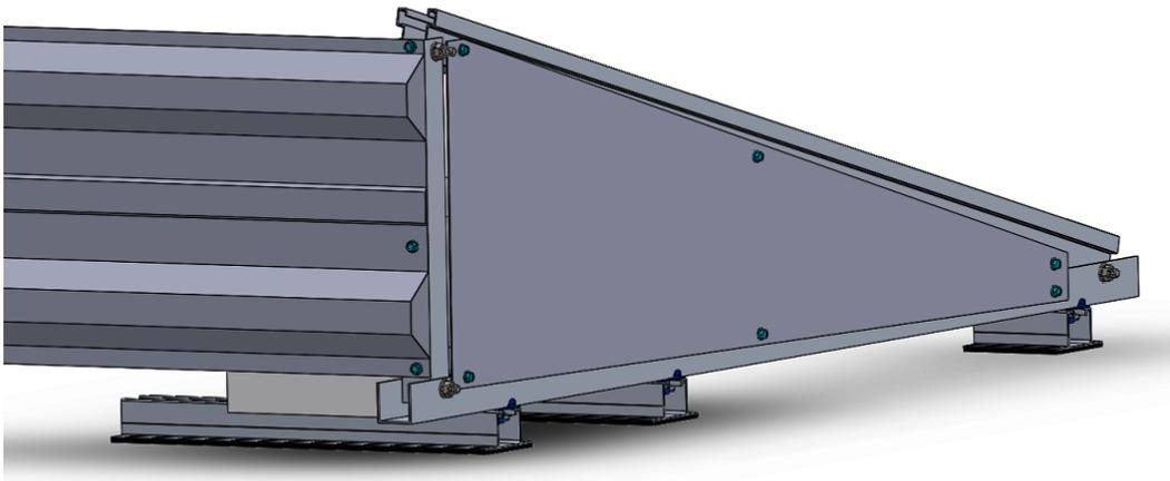
**STEP 5.- Longitudinal connection between profiles**
