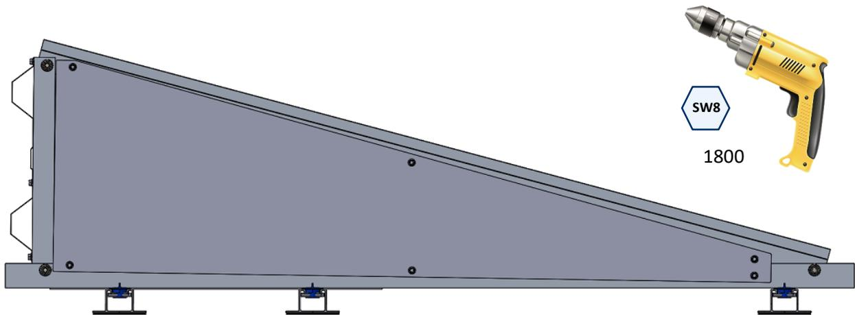
The back windbreaks are fixed with three self-drilling screws as shown in the picture.
