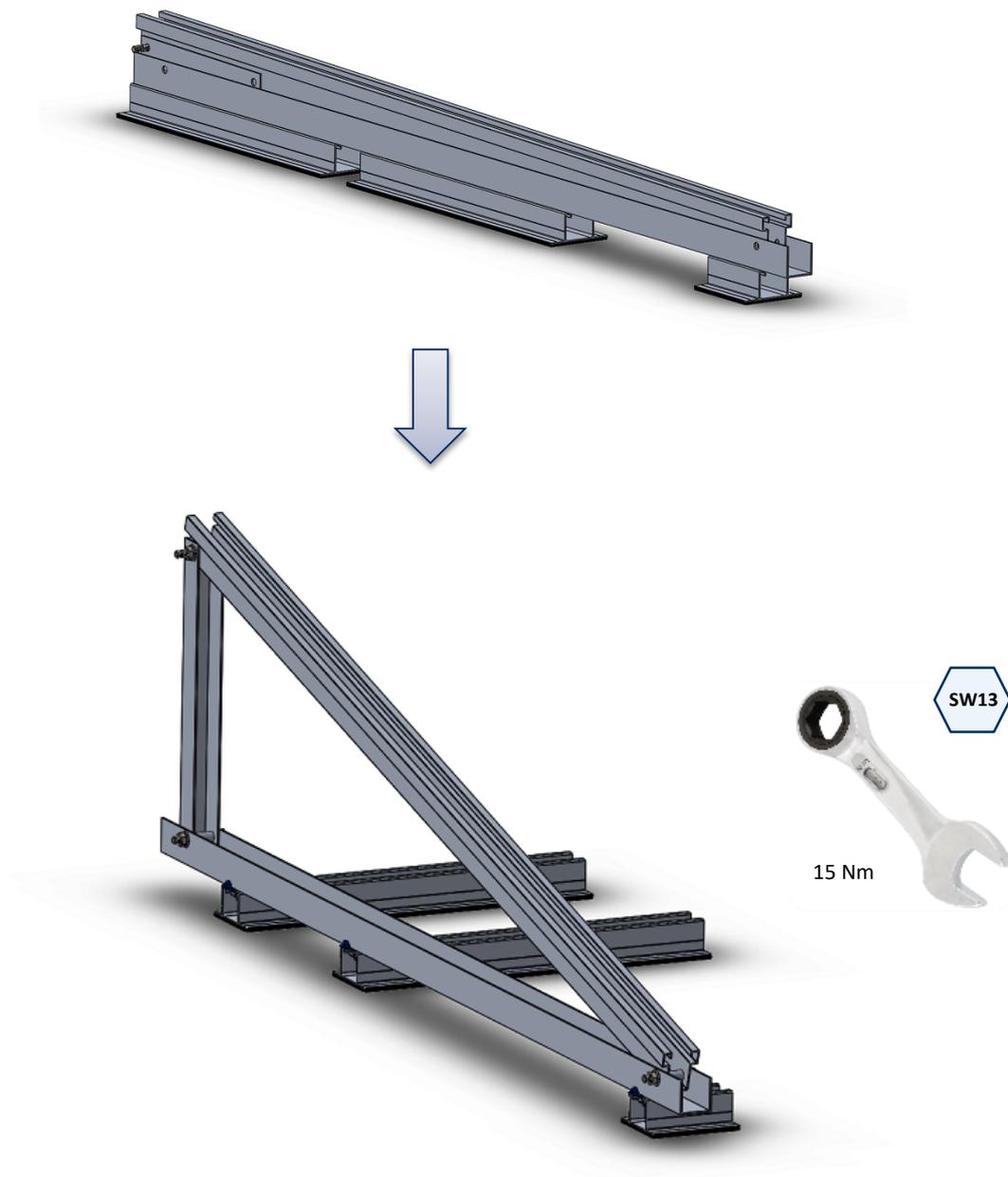
**STEP 3.- Mounting the side and rear windbreakers**
