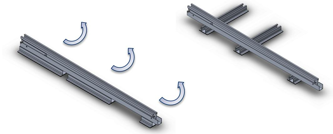
Position the support profile at 90° with respect to the lower profile, insert the stainless steel screw through both profiles placing a bushing so that when applying the tightening torque the profiles do not deform and finally place the stainless steel nut at the other end and apply a tightening torque of 15N/m.
