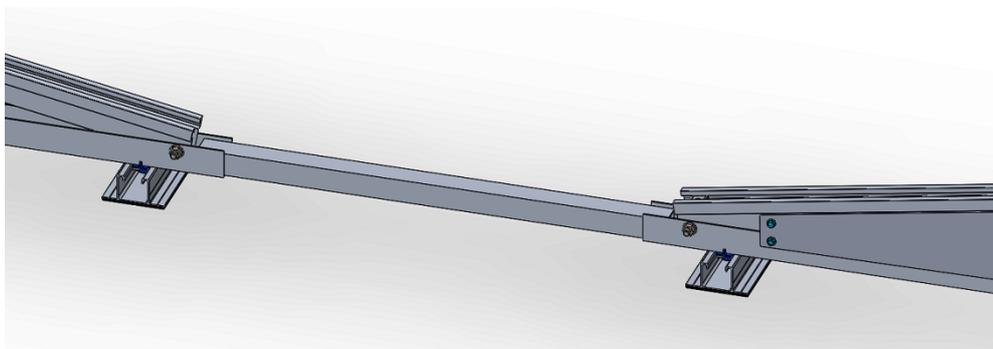
Fix the joining profile to the lower profiles by installing 2 stainless steel self-drilling screws on each side. The screws must be installed on the sides of the profile, in the shape of a cross so that they do not collide with each other. For the installation of the screws, an electric screwdriver equipped with a SW-8 hexagonal socket is needed, an installation speed of 1800 rpm is recommended.
