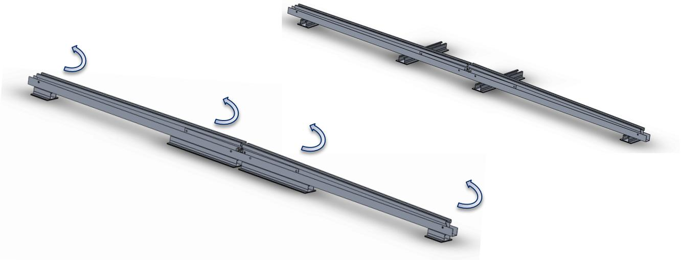
Position the support profile at 90° with respect to the lower profile, insert the stainless steel screw through both profiles placing a bushing so that when applying the tightening torque the profiles do not deform and finally place the stainless steel nut at the other end and apply a tightening torque of 15N/m.
