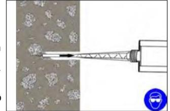
6. Insert the mixer nozzle (resin stopper / extension tube if applicable) to the bottom of the hole. Begin to extrude the resin and slowly withdraw the mixer nozzle from the hole ensuring that there are no air voids as the mixer nozzle is withdrawn. Fill the hole to approximately 1/2 to 3/4 full and remove the mixer nozzle completely.
