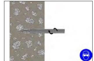
8. Any excess resin should be expelled from the hole evenly around the steel element showing that the hole is full. This excess resin should be removed from around the mouth of the hole before it sets.
