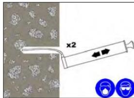
**If the hole collects water after the initial cleaning this water is recommended be removed before injecting the resin.**
