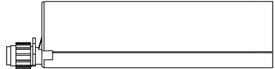
**Two part foil in a single piston component cartridge (FCC)**
