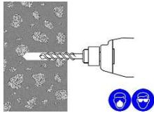
Drill hole to the required embedment depth using a hammer-drill with carbide drill bit set in rotation hammer mode, or a compressed air drill or diamond core drill.
