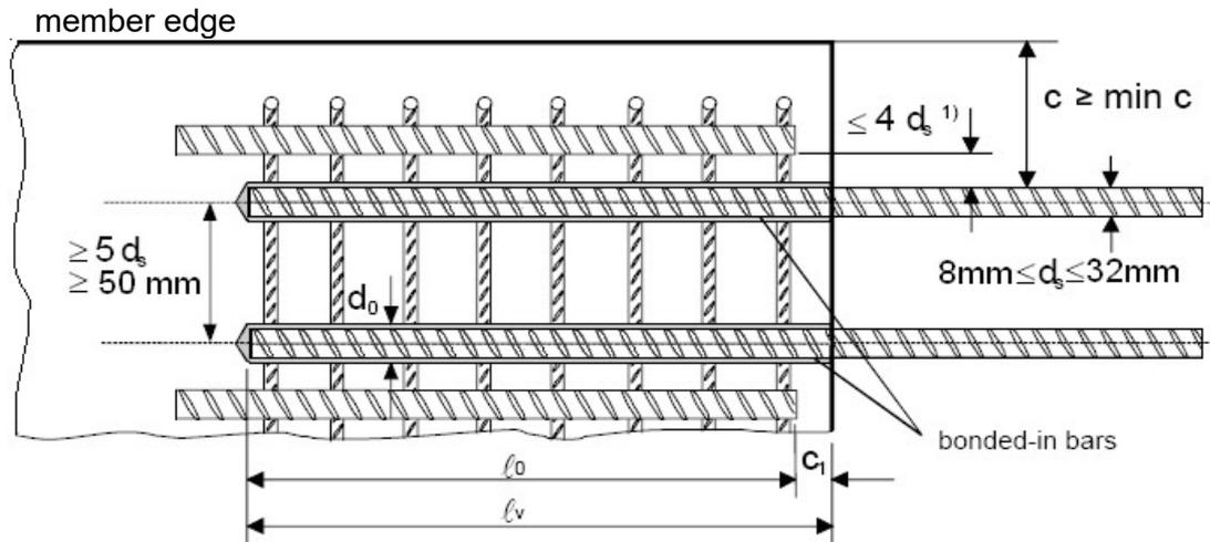
1) If the clear distance between lapped bars exceeds  $4d_s$  then the lap length shall be increased by the difference between the clear bar distance and  $4d_s$
