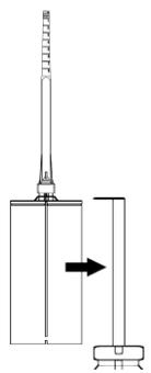
**Note:** The MORCAPUH nozzle is in two sections. One section contains the mixing elements and the other section is an extension piece. Connect the extension piece to the mixing section by pushing the two sections firmly together until a positive engagement is felt.
