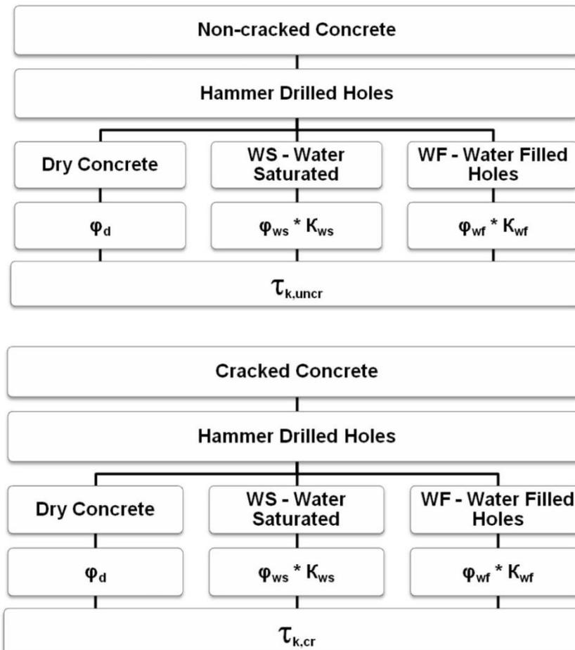
FIGURE 1—FLOWCHART FOR THE ESTABLISHMENT OF DESIGN BOND STRENGTH
